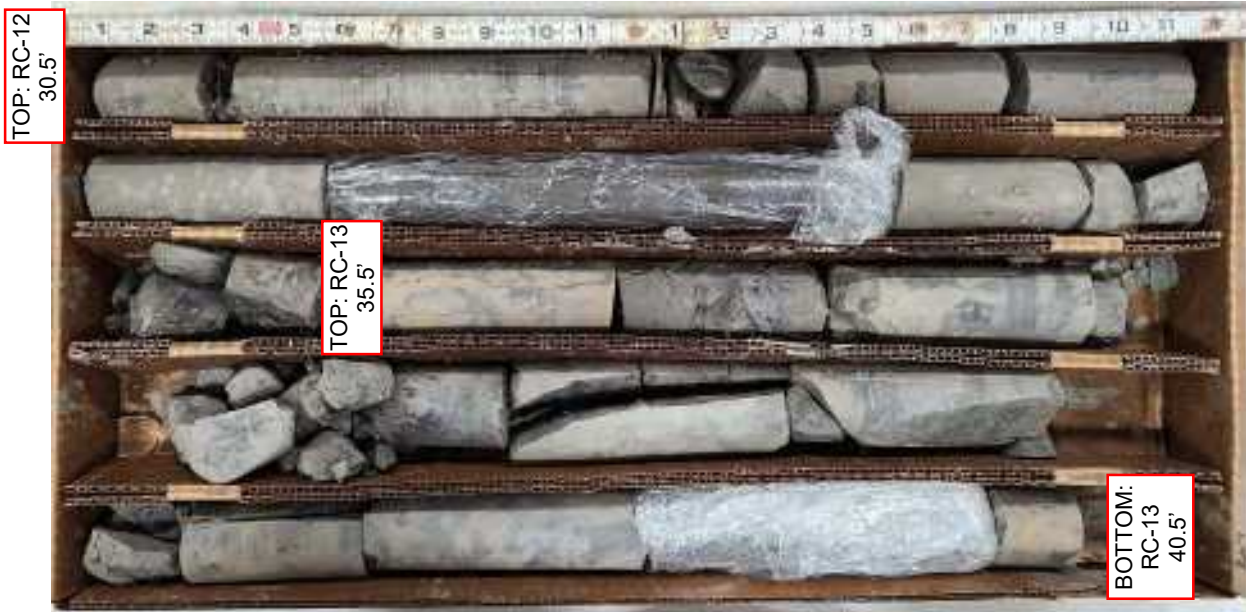
Rock Core Photograph 3. Boring B-103, Core Runs RC-12 and RC-13 (30.5 to 40.5 feet deep).
