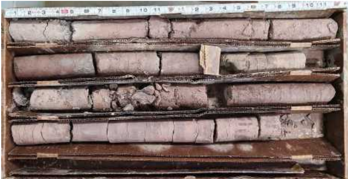
Rock Core Photograph 3. Boring B-3, Core Runs RC-7 and RC-8 (10 to 20 feet deep).
