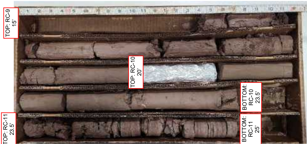
Rock Core Photograph 1. Boring B-101, Core Runs RC-9, RC-10, and RC-11 (15 to 25 feet deep).
