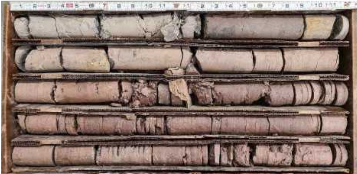
Rock Core Photograph 1. Boring B-1, Core Runs RC-10 and RC-11 (25 to 35 feet deep).
