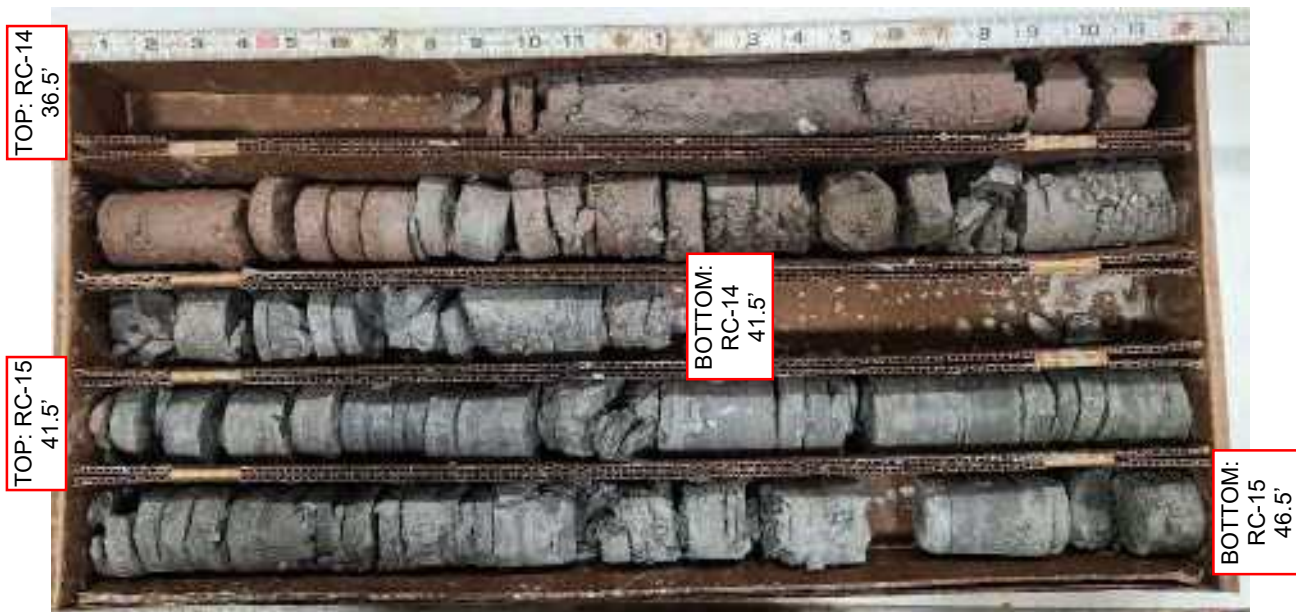
Rock Core Photograph 2. Boring B-102, Core Runs RC-14 and RC-15 (36.5 to 46.5 feet deep).
